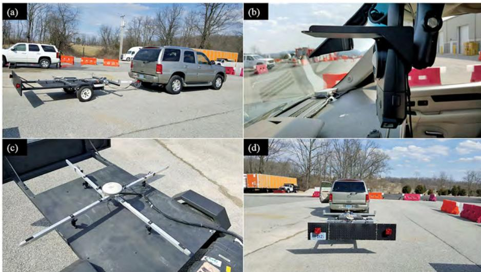
Figure 2. TRLMMS developed at VTTI: (a) TRLMMS hitched to vehicle; (b) Illuminance meter that measures the vertical illuminance mounted to the windshield; (c) "Spider" apparatus with GPS unit in the center; and (d) TRLMMS from behind with the headlamp barrier eliminating the influence of the following vehicle's headlamps.
